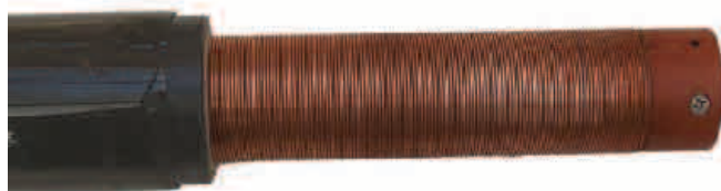
Figure 6 — Exposed coil in the screwdriver antenna.
